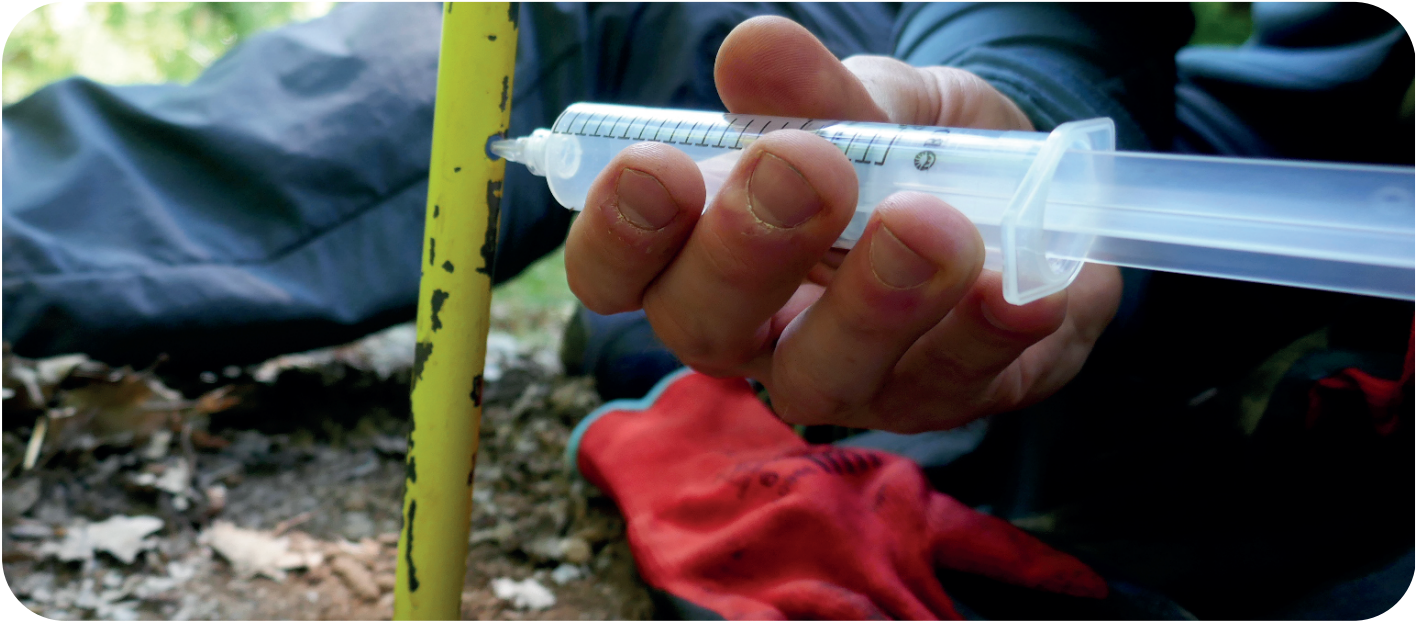
45-8 ENERGY - Taking a near-surface gas sample during a field campaign.
